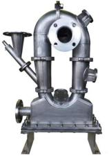
The loop jet mill is designed with an inverted trapezoidal shape, which forces the circulating particles to concentrate at the nozzles. These rapidly moving particles collide and rub against each other, breaking
