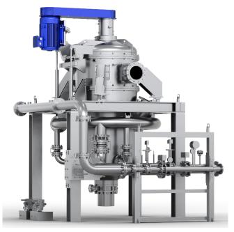
Driven by the high-speed air, the particles in a fluidized bed jet mill are accelerated and collide at the intersection point of the nozzle jets, thereby achieving the purpose of micronization.
